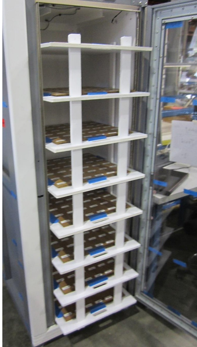
Figure 11. RFID Tag Fixture in the Tower Cabinet
