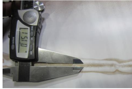
Figure 21 – Establish Roller Touch Width
