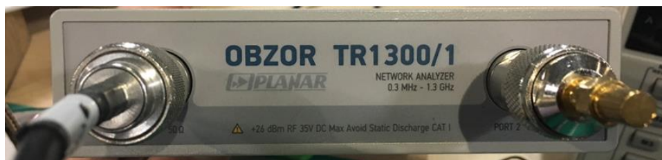
Figure 1 - Network Analyzer used in Manufacturing
