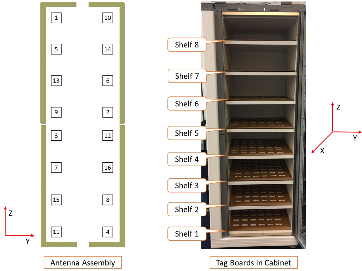
Figure 10. Tags in the Tower Cabinet
